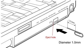
Figure 4-27 Manual release with the eject hole
